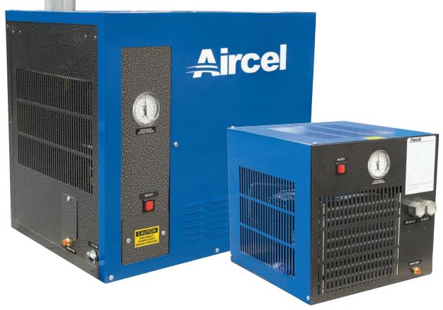
The Aircel **DHT Series (20 - 125 scfm)** high inlet temperature refrigerated air dryers are designed for air-cooled, reciprocating type air compressors. This compressed air dryer combines an oversized refrigerated circuit, high-efficiency heat exchangers, and separator into a single compact unit. Also includes single point air in/out, drain, and electrical connections.
