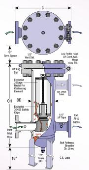
Series R40 coalescing pipeline filters are fabricated from rugged enameled carbon steel, (R42 are 304SS), designed, constructed, and stamped in accordance with ASME Boiler and Pressure Vessel Code requirements for unfired pressure vessels. Any model can be modified to more exactly
