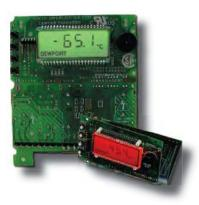
Model XDT-OEM is a stand alone board suitable for mounting in existing enclosures. Connections are made through a pluggable screw terminal block which allows cables to leave the board vertically or horizontally.
