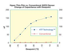
this change is quasi linear and its sensitivity to temperature is negligible. The advantages of a linear high capacitance response are: better sensitivity, better repeatability and
